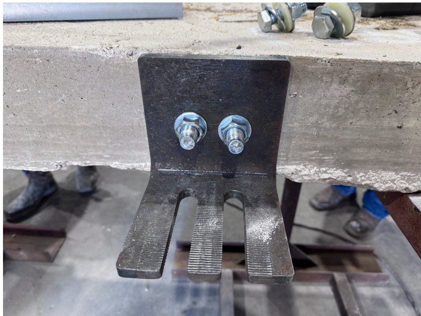
Photo No. 2 Connector Mounted to Concrete Slab
