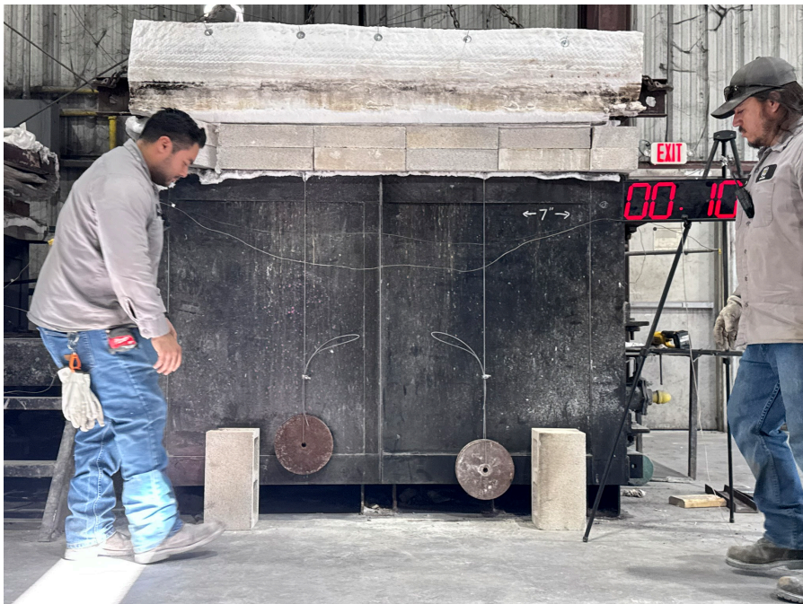
Photo No. 10 Connector Disengagement during Test 1
