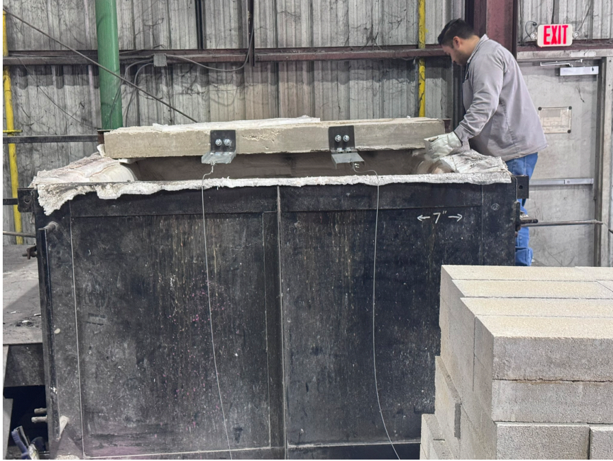
Photo No. 7 Steel Wire Connected to U-Channel
