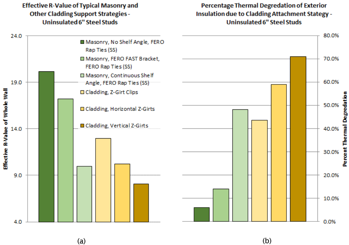
Figure 11. a) Effective R-value and b) corresponding percent thermal degradation of typical masonry veneer and other cladding support strategies using 4 inches of exterior insulation over uninsulated 6-inch steel studs
