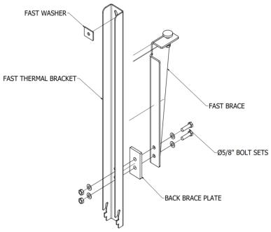
The Back Brace Assembly prevents deflection by providing support when the FAST Thermal Bracket<sup>™</sup> offset shelf angle support ("FAST Thermal Bracket") exceeds 25" in height.
