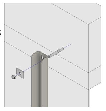
2. Temporarily install all FAST Thermal Brackets along a line of shelf angle to level the shelf angle. Mark the location of the Back Brace connection once everything is level.
