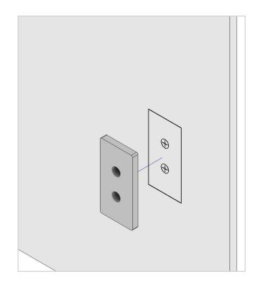
4. Install the Back Brace plate in the cutout of the sheathing and reseal the air vapor membrane on the surface of the back brace plate. Fasten the FAST Thermal Bracket to the Back Brace plate.
