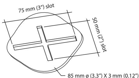
Figure 2 Insulation Support/Retainer
