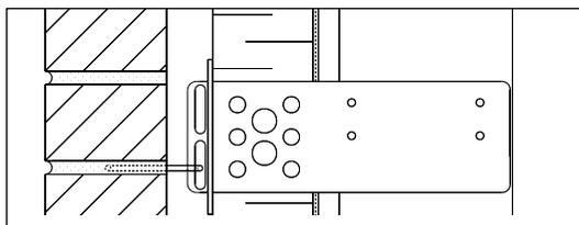
Figure 5 Slotted Stud Tie (Type II) Installed
