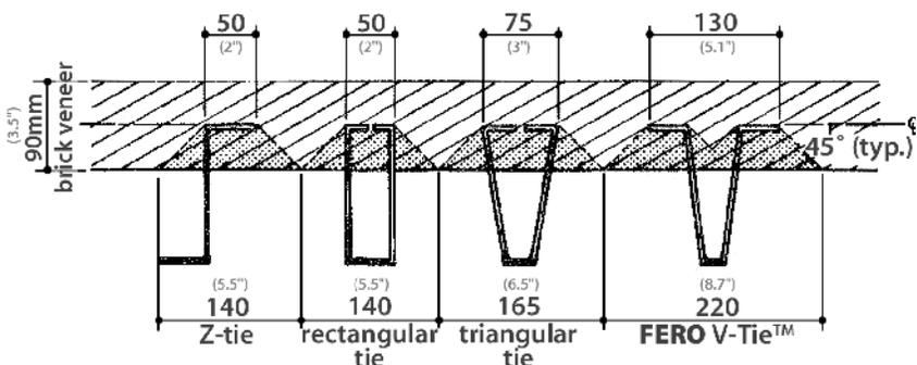
Figure 4 Effective Mortar Joint Area Pullout Resistance
