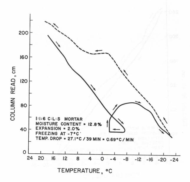
FIGURE 3 - VOLUME CHANGE DUE TO FREEZING
