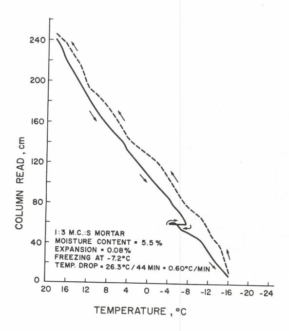
FIGURE 4 - VOLUME CHANGE DUE TO FREEZING
