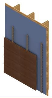
The FERO Vented Furring Strip creates a vented rainscreen channel between the building wrap and the siding material, creating a durable and rigid connection between the siding and the backing material. With a drainage channel behind the siding, any wind driven or incidental water that penetrates the siding layer is easily drained by gravity or air vented through evaporation away from the building
